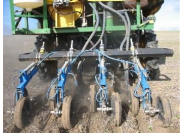
Prarie application w/deep banding machinery Source: biocharapplication.com
